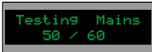
Next the mains frequency is tested, to determine if you have 50 Hz or 60 Hz mains.
