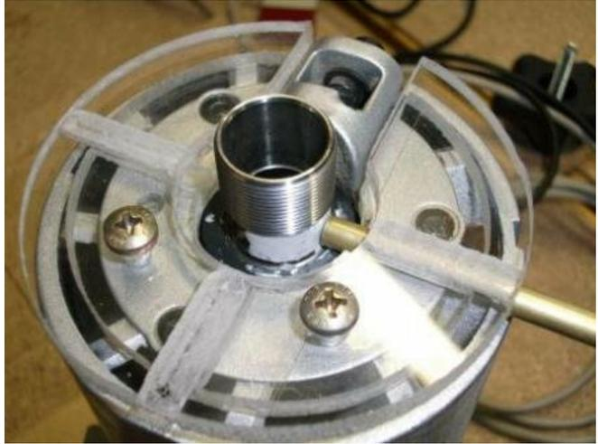
Here are some spindle RPM sensor mountings, at the top or bottom of the router.
